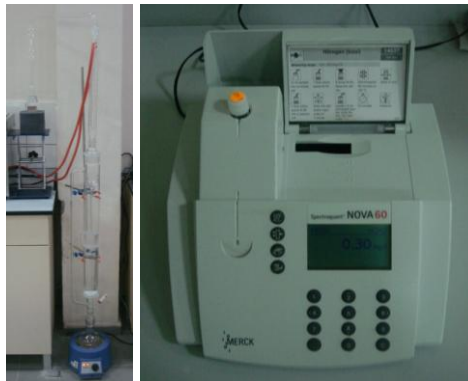
Fig. 3 Formaldehyde Emission Test Set-up (Photo: Candan)
