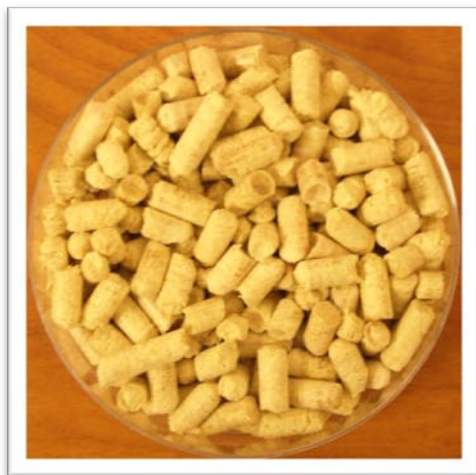
Figure 1 The bamboo pellets with 16% MC and PS mixture
