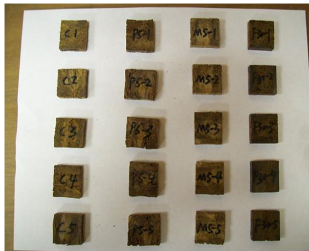
Figure 8 Block appearance for untreated and treated PSL after 28-day termite test
