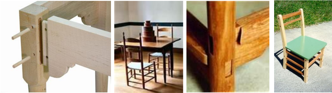
Figure 3. Shrink and swell joinery examples used in Shaker's furniture, oriental furniture and school furniture.
