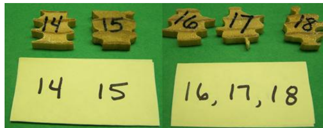
Figure 7 Block appearance for southern pine positive control after 28-day termite test
