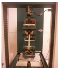
Fig. 1 Machine and test specimens according to EN302-1
