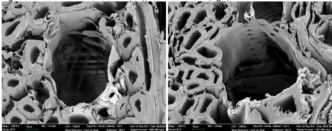
Fig 5. Cell wall of air-dried wood(left) and heat-treated wood(right)
