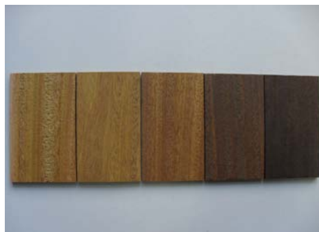
Fig.2. The color of heat treatment and control test specimen
